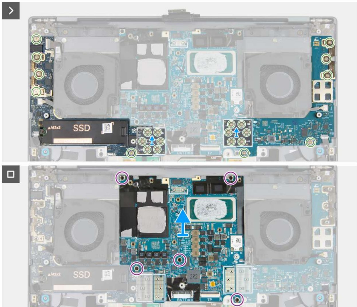
Figure 51. Removing the system board (integrated graphics)
