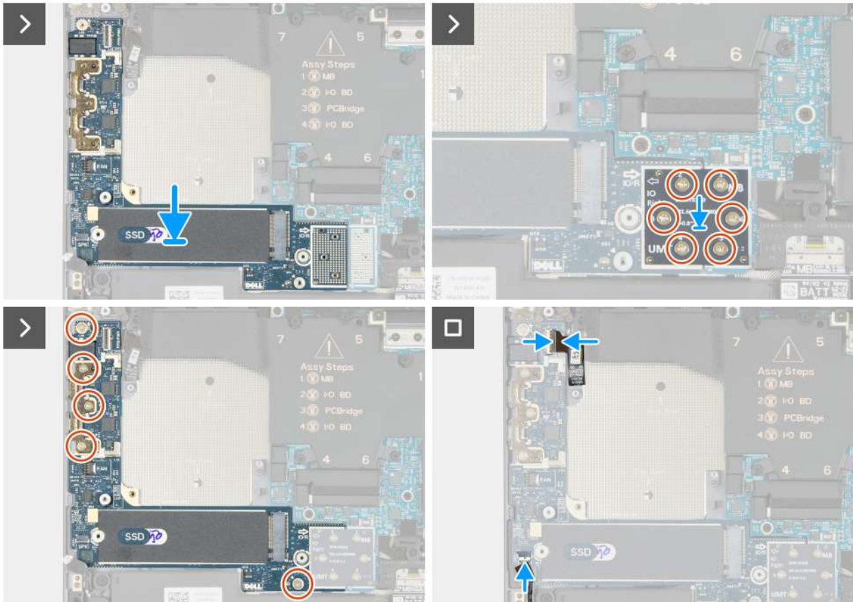
Figure 48. Installing the right I/O-board
