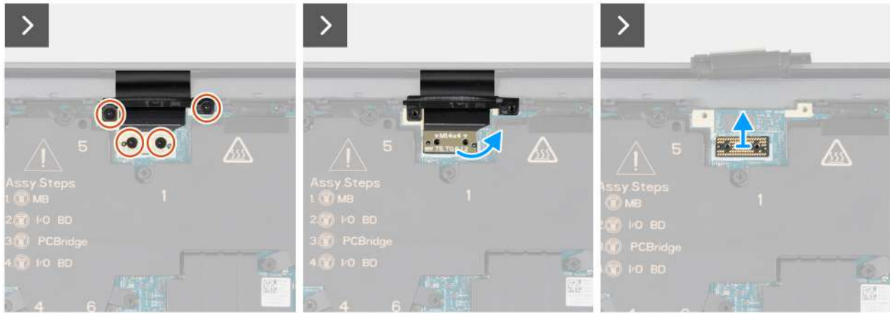
Figure 31. Removing the display assembly
