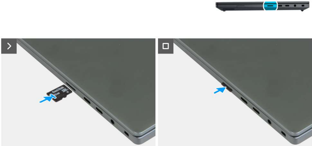
Figure 11. Installing the memory card
