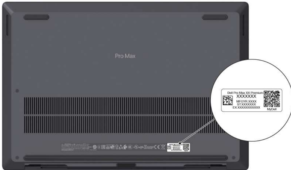
Figure 7. Service Tag/Express Service Code location
