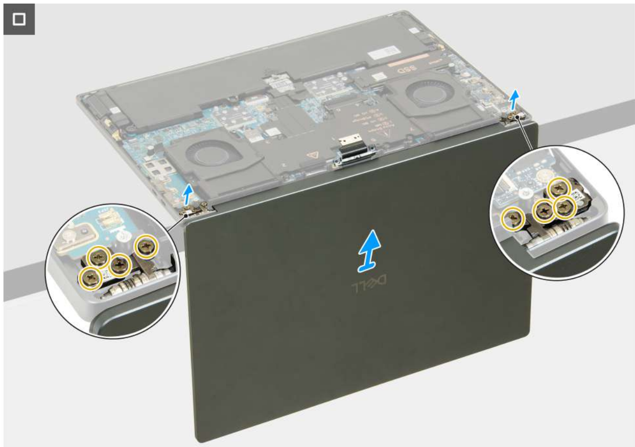
Figure 32. Removing the display assembly
