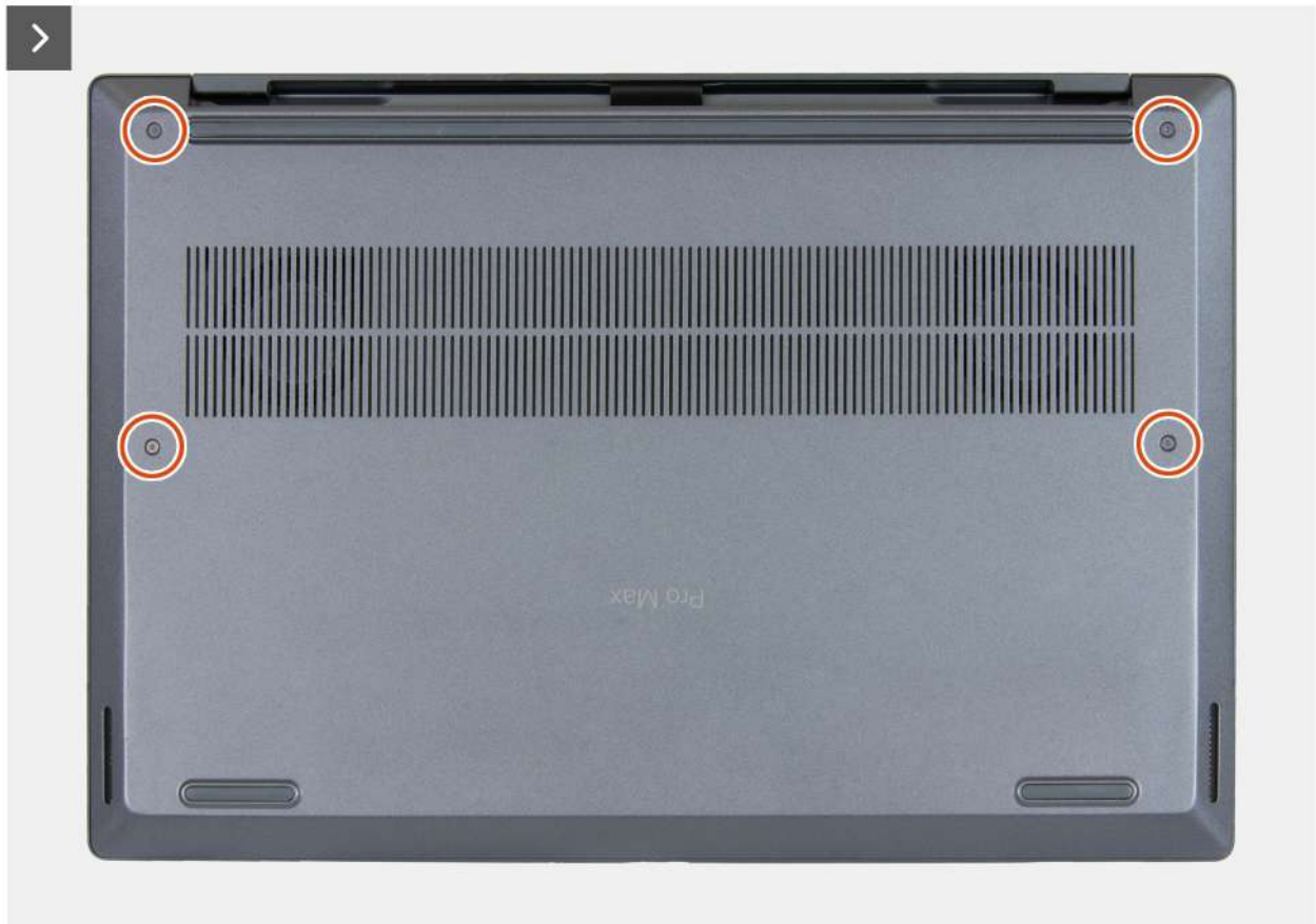
Figure 12. Removing the base cover
