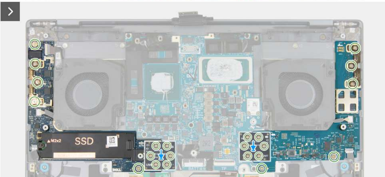
Figure 63. Installing the system board (discrete graphics)
