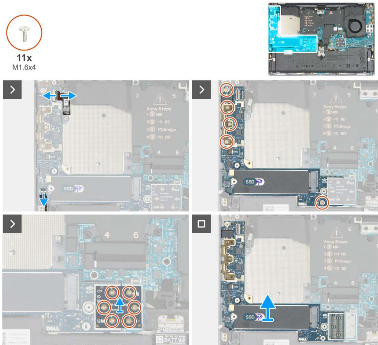
Figure 47. Removing the right I/O-board
