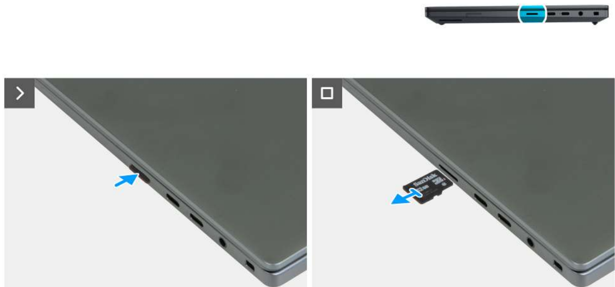
Figure 10. Removing the memory card
