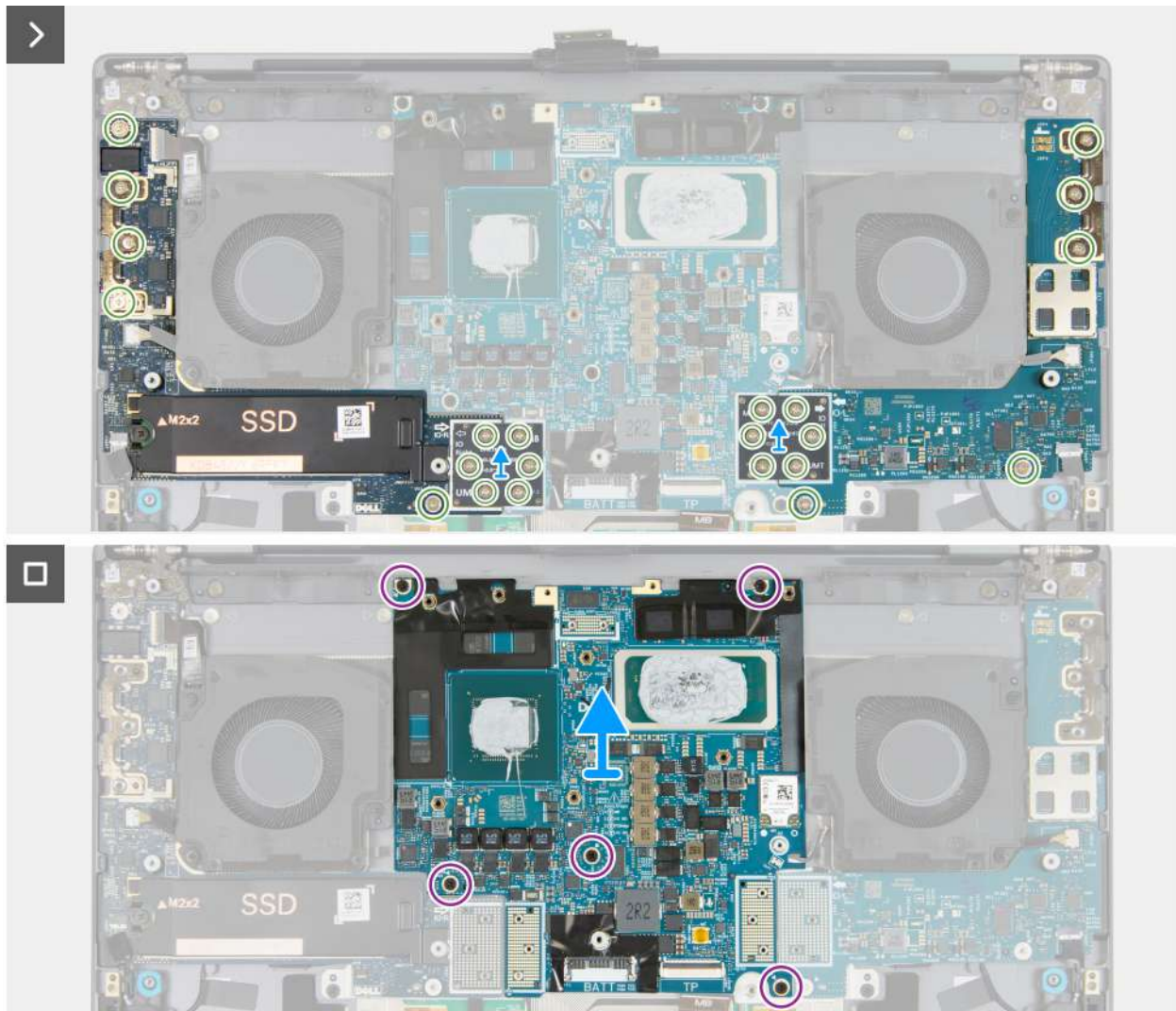
Figure 60. Removing the system board (discrete graphics)
