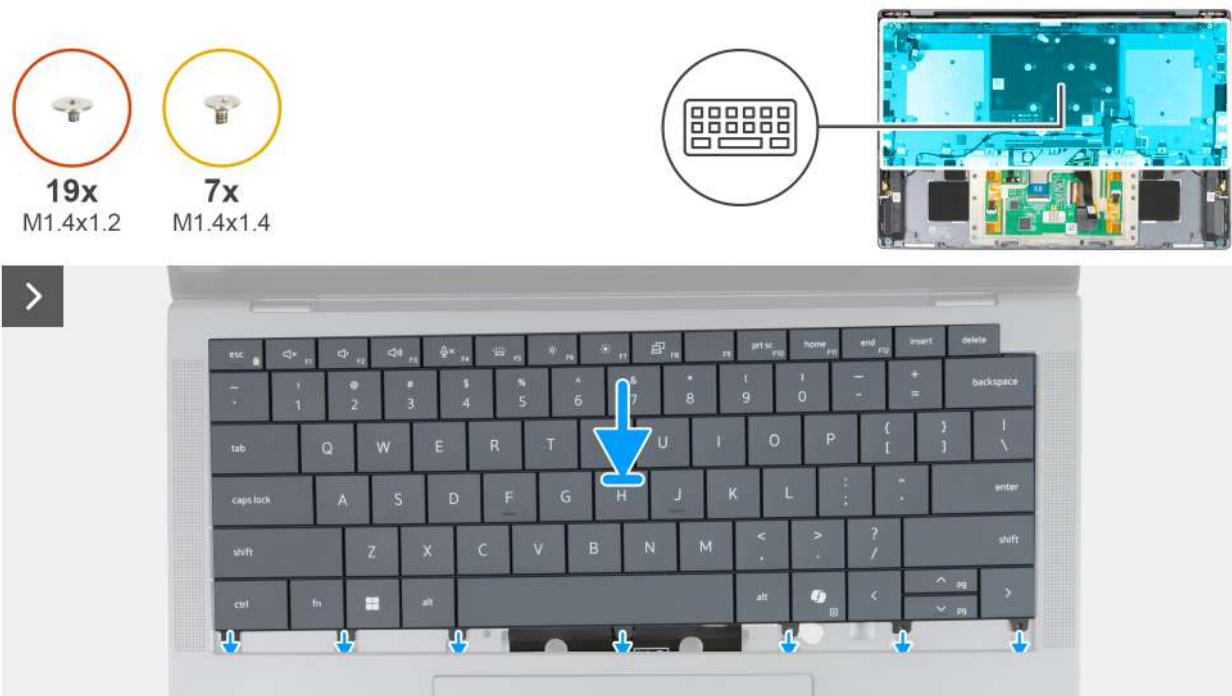
Figure 74. Installing the keyboard
