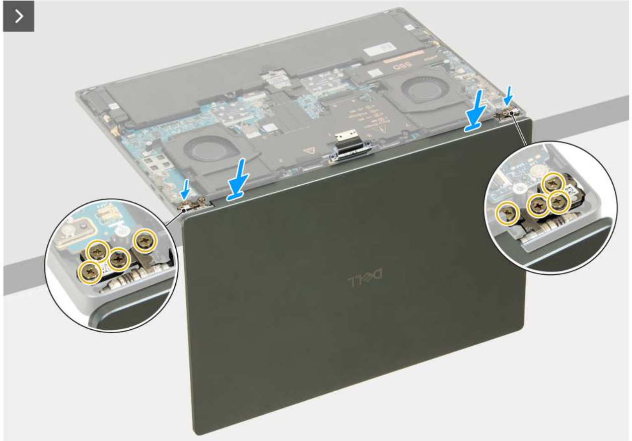
Figure 38. Installing the display assembly
