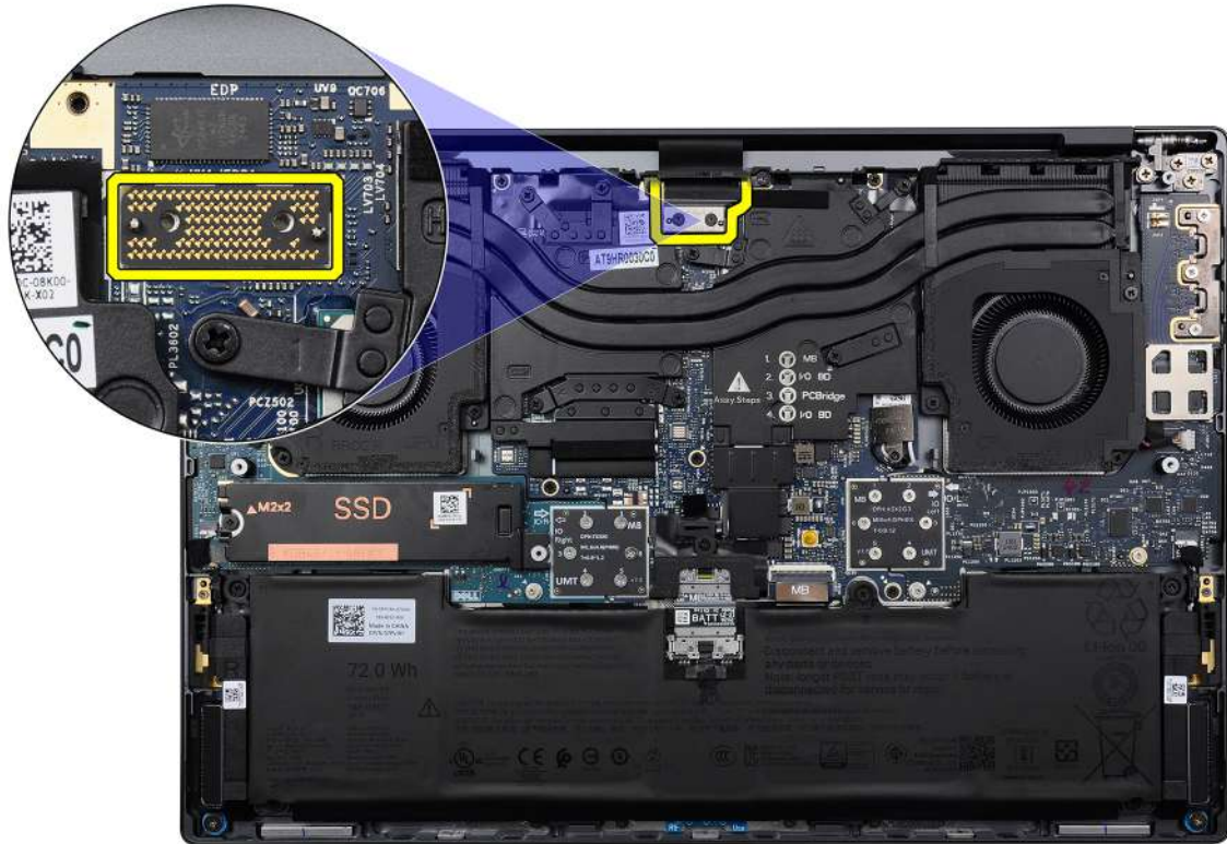
Figure 35. Display-assembly cable interposer board
