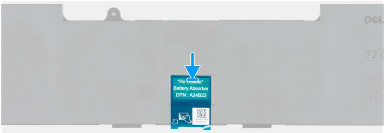
Figure 20. Installing the battery absorber
