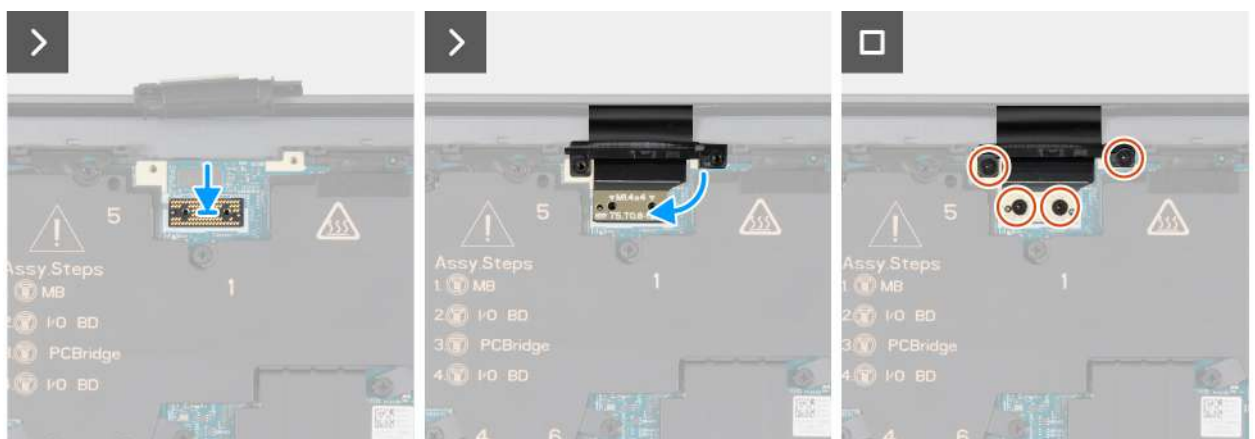
Figure 39. Installing the display assembly
