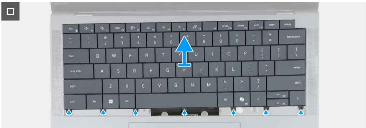
Figure 72. Removing the keyboard
