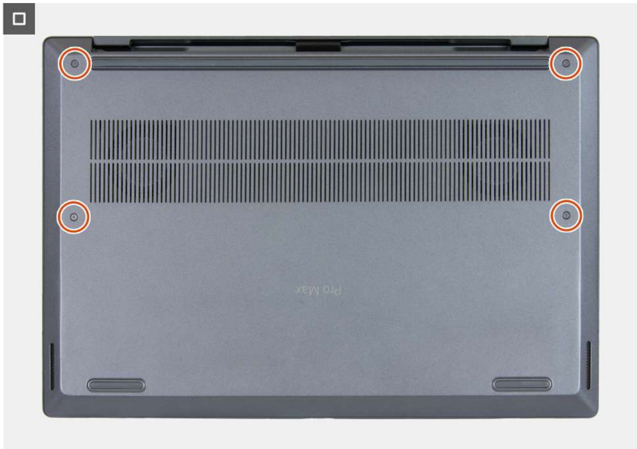
Figure 15. Installing the base cover
