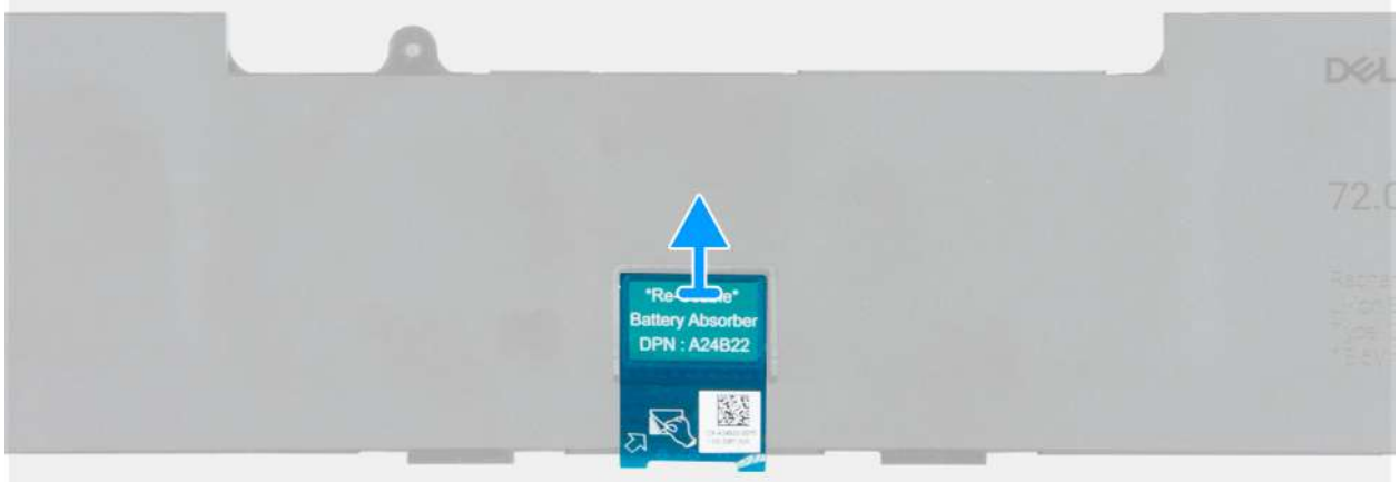
Figure 18. Removing the battery absorber
